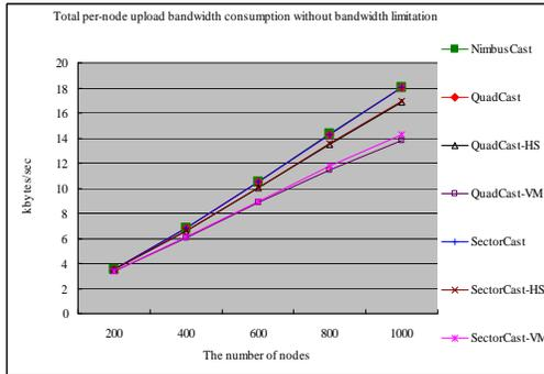
Figure 10. Total per-node upload bandwidth consumption without bandwidth limitation for AIO voice chatting schemes
