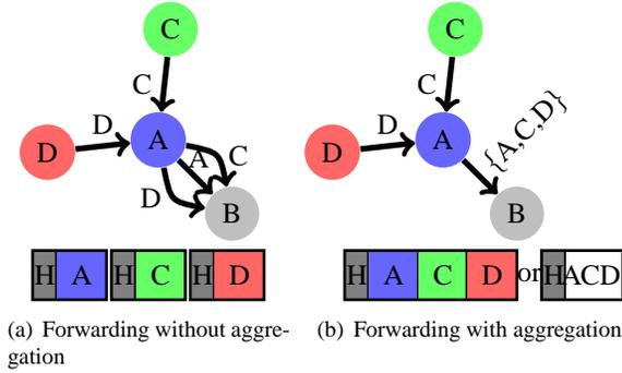
**Figure 7. Examples of packet aggregation**
