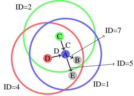
**Figure 8. The concept of packet aggregation by 2-power number addition**
